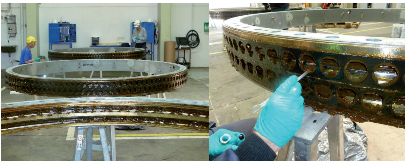
Figure 4: Representative reference grease sampling from a dismantled 3.6 MW blade bearing. Increments from every second ball support hole were used for 3-D heterogeneity characterization of the grease in the complete 360 degree active zone in the space between the raceways. This is a 1-to-1 match analogue to “stopped belt” sampling in conventional PAT.
