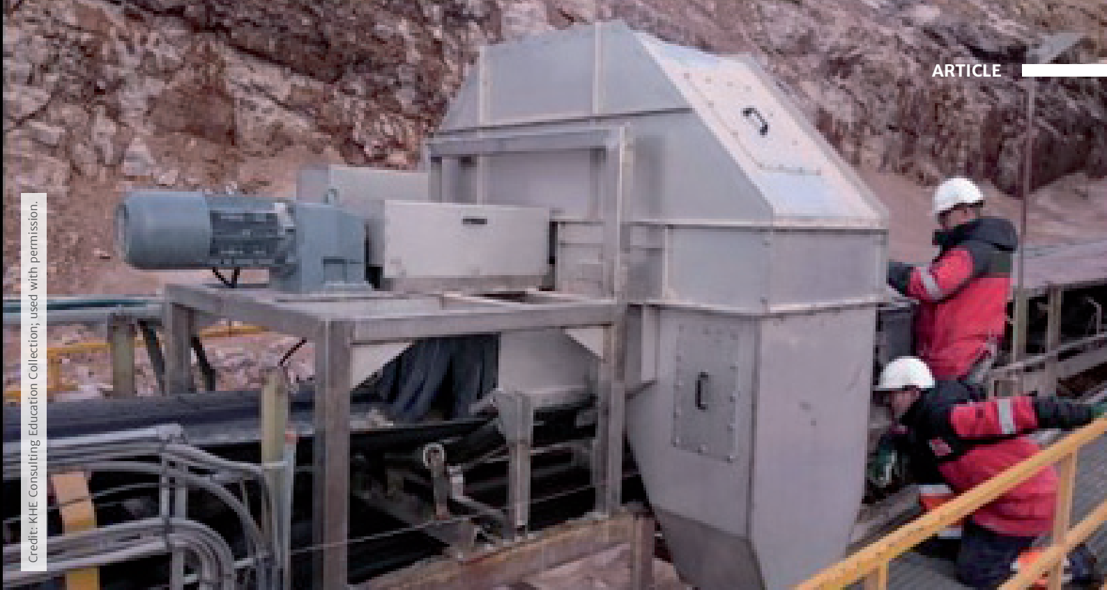
Figure 4: Anonymised illustration of a particularly popular type of cross-belt sampler, the hammer sampler. For very many designs, brands and implementation this type of equipment cannot deliver a representative cross-belt cut, as extensively described, documented and warned against in the TOS literature [2,3,5]. Caveat: this example is meant for illustration of principles only; no identification of company, personnel or equipment brand is intended.
