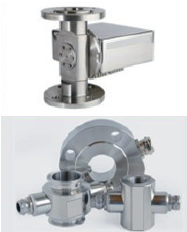
Figure 5: Examples of process sampling interfaces (PSI) designed to be installed as part of ducted flow. Note how flanges allow flush implementation in pipelines, while offering openings and fixtures allowing to project sensor radiation orthogonally across the material flow a.o. Caveat: these examples are meant for illustration of principles only; no identification of company or equipment brand is intended.
