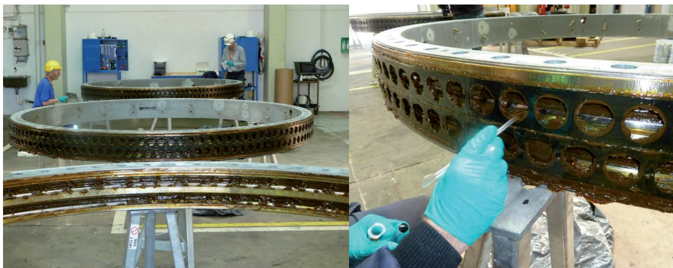
Figure 4: Representative reference grease sampling from a dismantled 3.6 MW blade bearing. Increments from every second ball support hole were used for 3-D heterogeneity characterization of the grease in the complete 360 degree active zone in the space between the raceways. This is a 1-to-1 match analogue to “stopped belt” sampling in conventional PAT.
