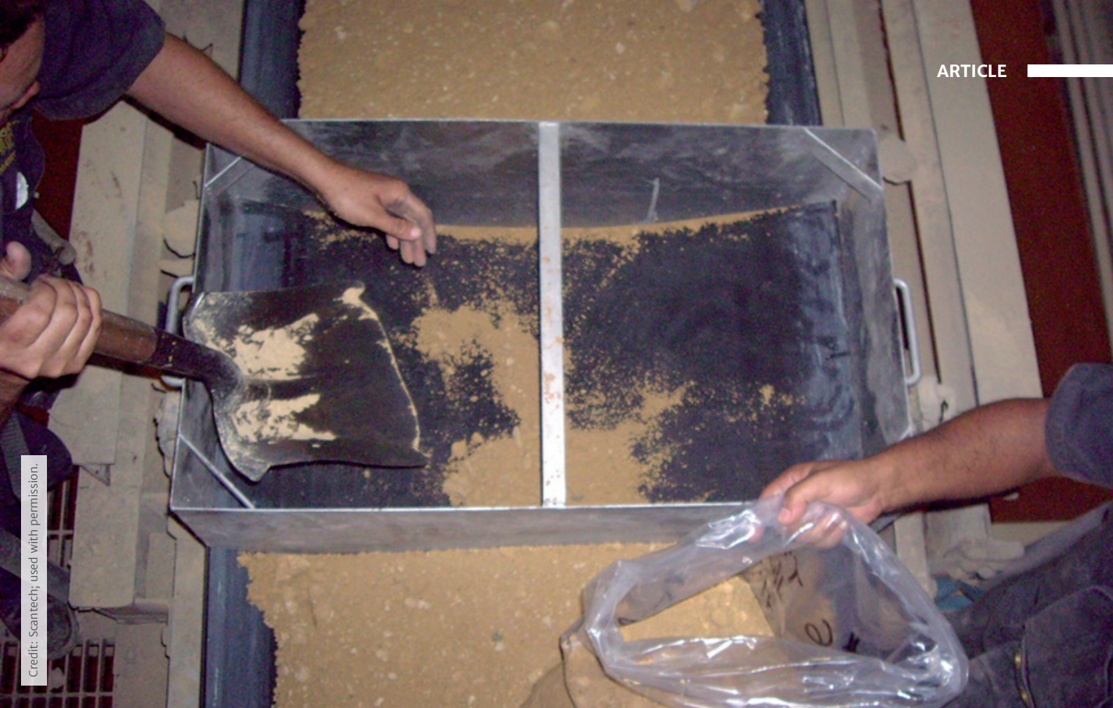
Figure 6: Example of stopped belt sampling to remove a stream cut from a conveyed flow as fully as possible to compare with PAT measurement data from the same segment to reference laboratory assay results.
