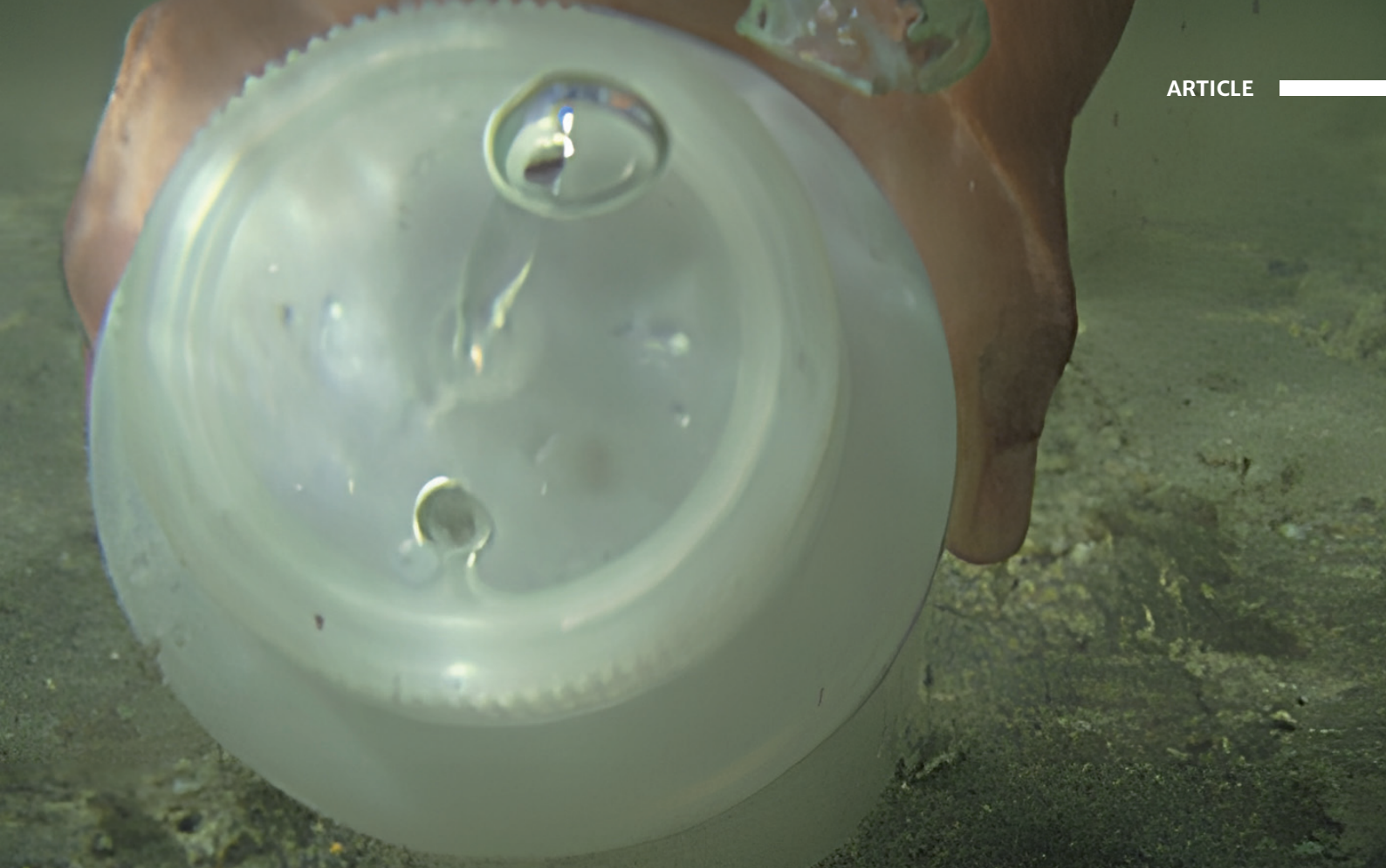
Figure 6: The Aloha Sampler in operation. Note air bubble leaving the upper hole in the aperture cover.
