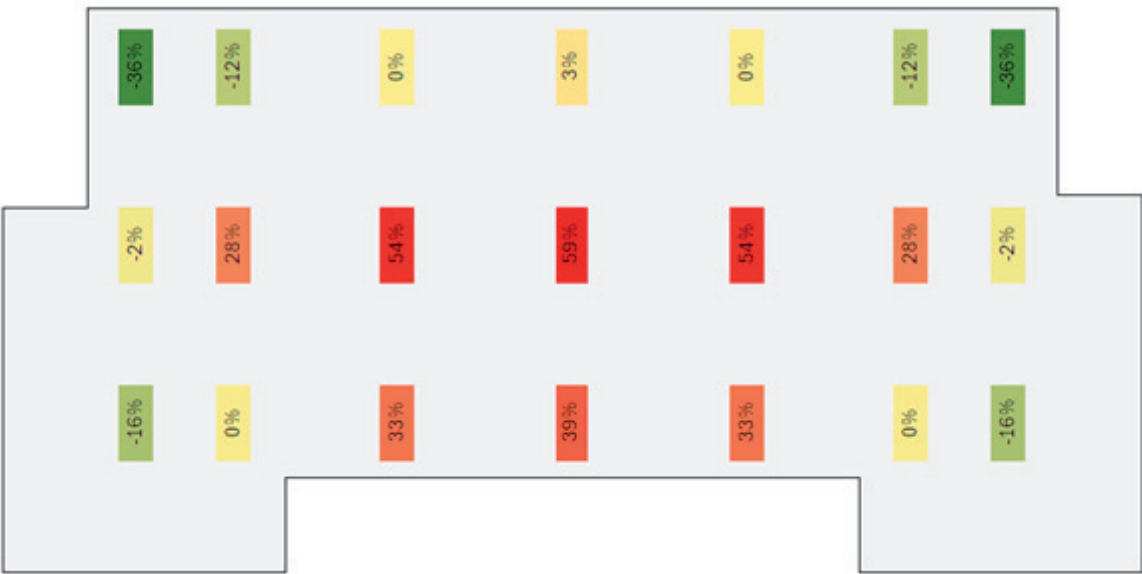
Figure 6: Cross-sectional heat map depicting the relative weight given to specific locations of the jar in determining their gold grades by PhotonAssay. Due to the random rotational orientation of the jar about its axis of rotation during analysis, there is no differentiation between the sides of the heat map, and the diagram is symmetrical.
