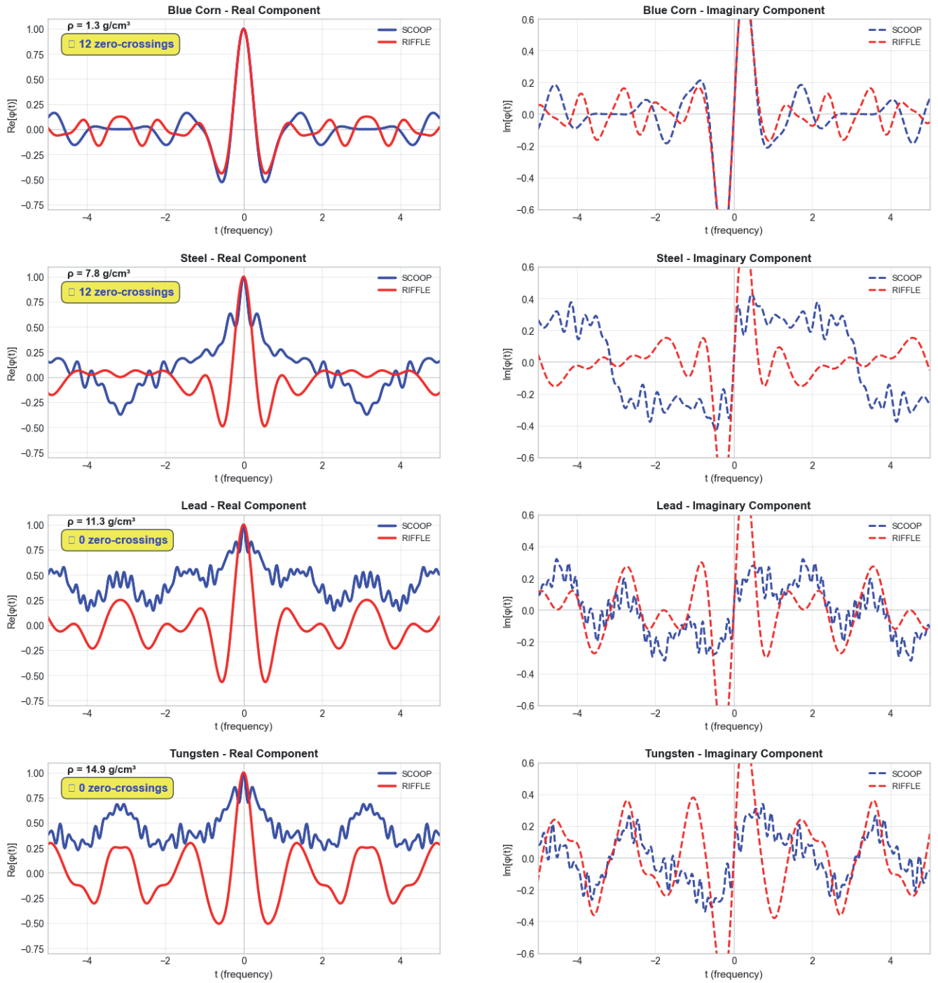
Figure 7: Empirical Characteristic Function comparisons for individual density tracers. The number of zero-crossings in the real component over t \in [-5, +5] provides a quantitative measure of distributional complexity. Each row corresponds to a tracer with increasing density ( \rho ) from top to bottom. Left panels show the real component Re[\varphi(t)] ; right panels show the imaginary component Im[\varphi(t)] . SCOOP method CFs (blue lines) exhibit increasingly complex oscillatory behaviour with particle density, while RIFFLE sampling distributions (red lines) show smooth, Gaussian-like decay across all tracers, indicative of consistent, unimodal sampling distributions.
