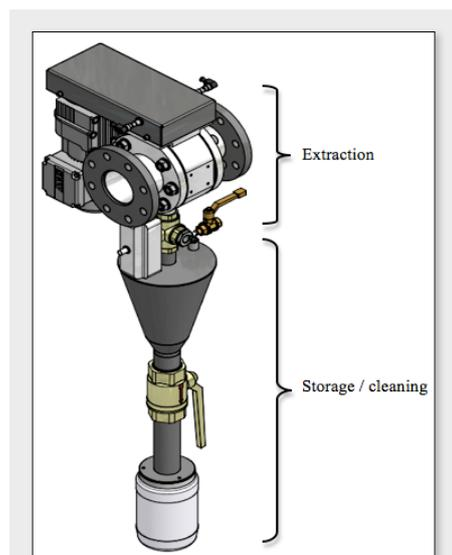
**Figure 1.** Schematic overview of the EF-sampler. Upper part shows the extraction mechanism including electric power supply and extraction mechanism with enclosed sampling arm. Lower part represents the storage/cleaning section including composing cylinder, pressure valve, storage valve and storage container.
