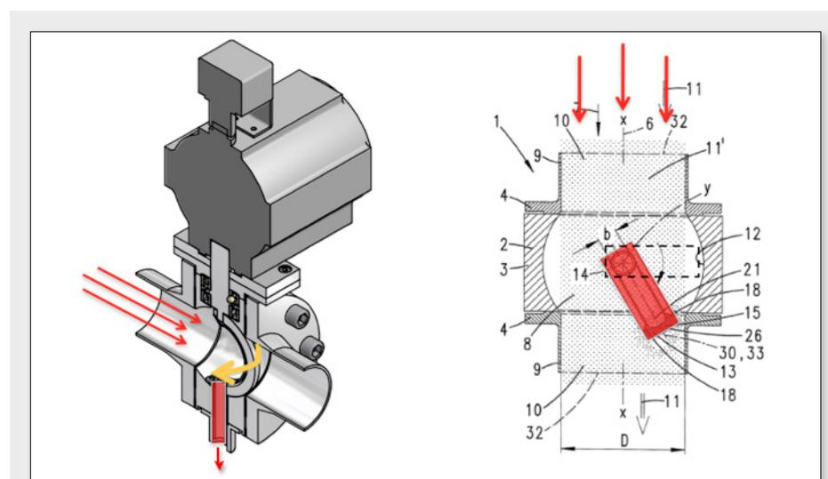
**Figure 2.** Schematic overview of the EF-sampler. Left figure showing side view, illustrating material flow direction, rotational movement of cutter arm and recovery of extracted material through outlet chute. Right figure shows top view of sampler, highlighting the rotational movement of the sampling arm, ducted material flow direction (top arrows) and parking position of sampling arm (dashed line).
