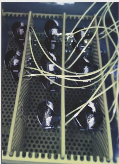
**Figure 4.** Training a “school” of bivalves in Biota Guard’s water exposure tank. Signal acquisition is otherwise reminiscent of PAT and is further processed by chemometric methods. Training can be simple employing only one parameter at a time, or more realistically, targeted on several interacting parameters in order to reach full compliance with the natural open sea characteristics at a target location.
