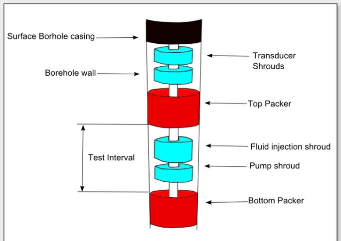
**Figure 2.** Multifunction BAT<sup>3</sup> in a bedrock borehole with borehole packers inflated to seal against the borehole wall (adapted from Reference 13).
