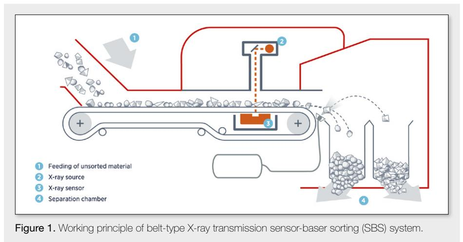
Figure 1. Working principle of belt-type X-ray transmission sensor-based sorting (SBS) system.
