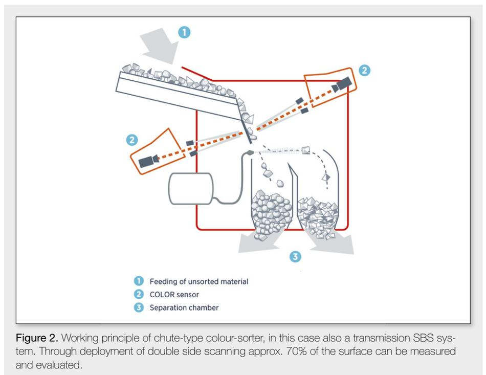
Figure 2. Working principle of chute-type colour-sorter, in this case also a transmission SBS system. Through deployment of double side scanning approx. 70% of the surface can be measured and evaluated.
