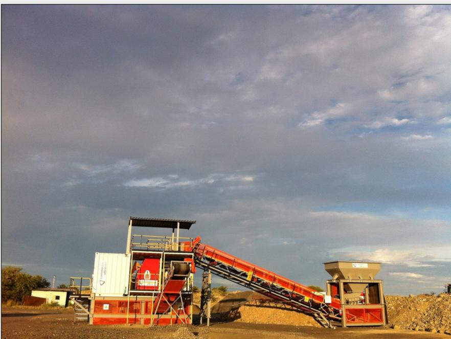
Figure 3. On-site containerised, semi-mobile chute-type sorter installation.
