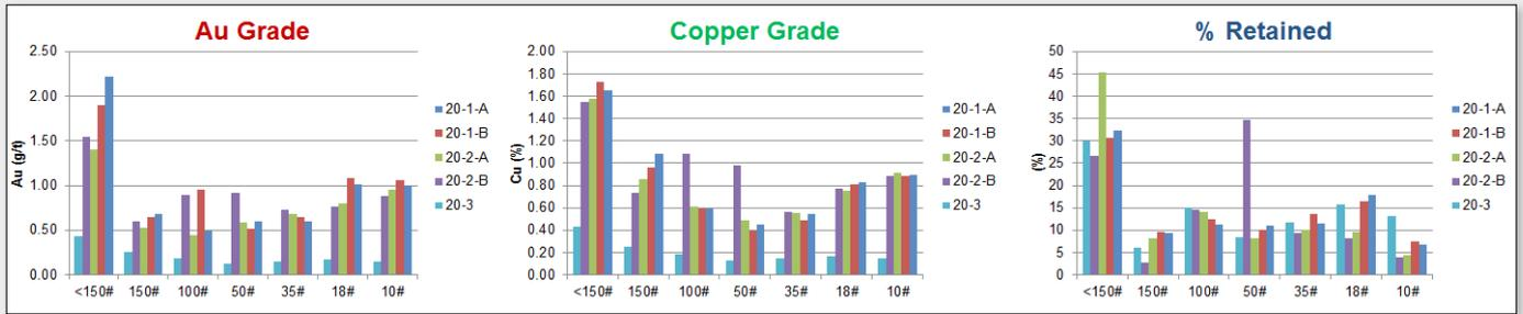
**Figure 5.** Gold and copper content by particle size fraction and percentage retained by particle size fraction. A and B samples as described in text. According to the Maraca Mine field sampling team, sample 20-3 originates from a part of the experimental block with distinctly lower ore grades, emphasising large fluctuations in the different regions of the block studied; sample 20-3 is therefore not immediately comparable to samples 20-1 and 20-2.
