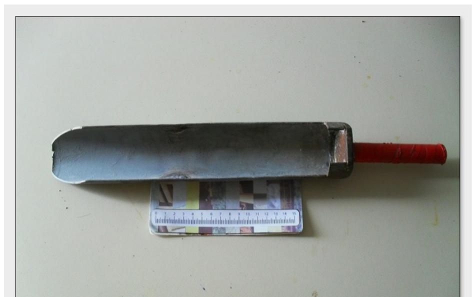
Figure 1. Shovel used for manual sampling.
