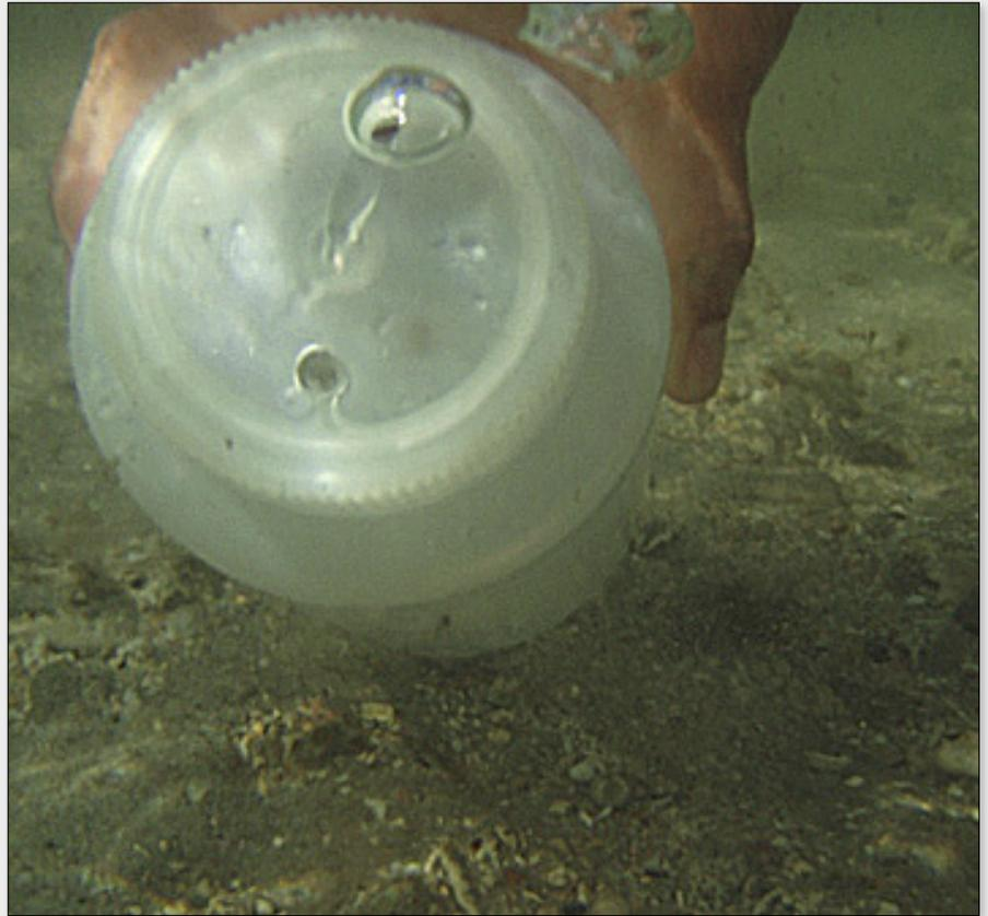
Figure 6. The Aloha Sampler in operation. Note air bubble leaving the upper hole in the aperture cover.
