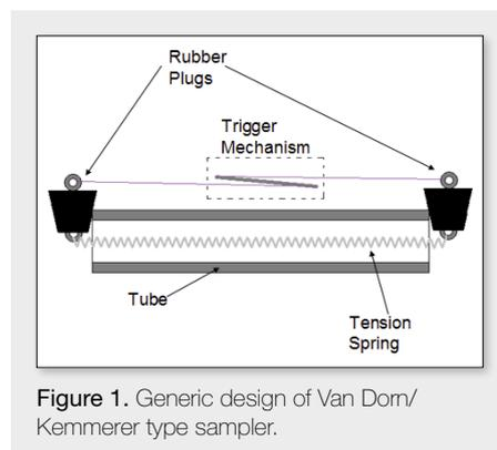
Figure 1. Generic design of Van Dorn/Kemmerer type sampler.
