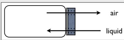
Figure 3. Basic operation of Aloha Sampler (Liquid Sampler Patent 7571657).
