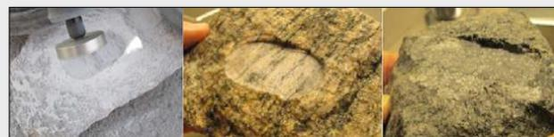
Improved surface hXRF fidelity resulting from application of the newly developed Field Rotary Abrasion Tool (FRAT)<sup>2</sup>
