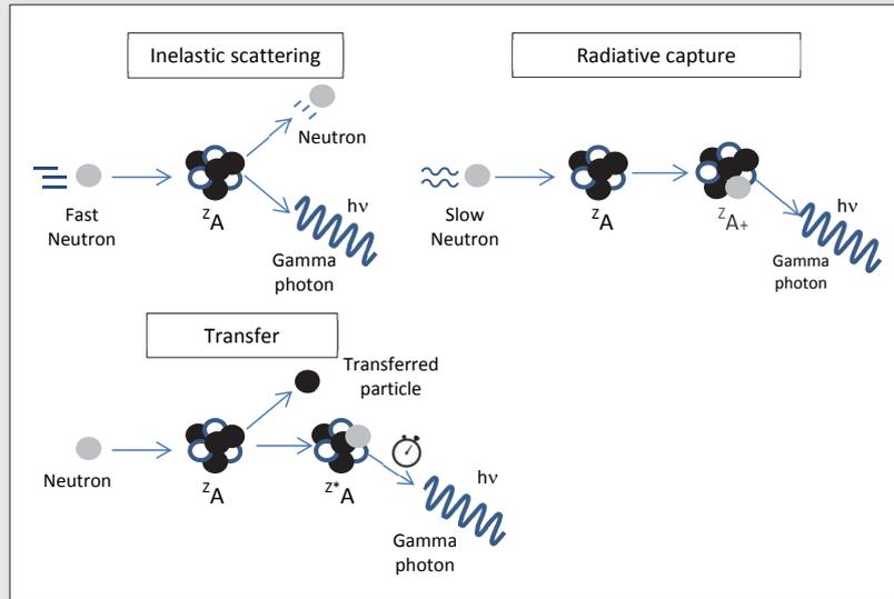
Figure 1. Neutron Interactions with matter
