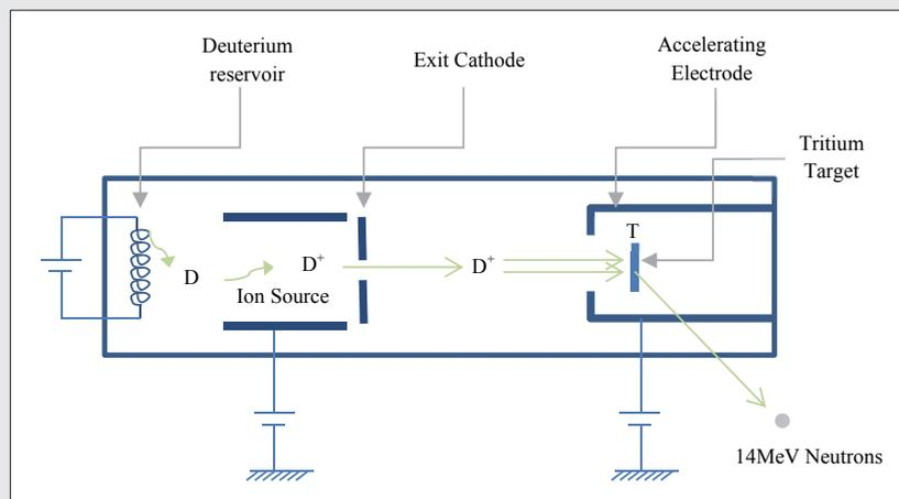
Figure 2. Neutron Tube Principle
