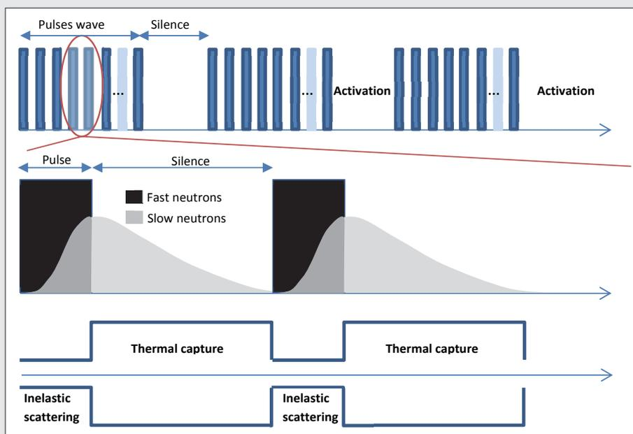
Figure 4. Pulse fast and thermal neutron analysis sequence
