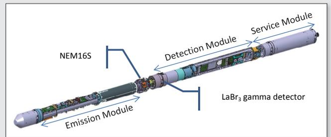
Figure 6. CAD view of the FastGrade™100 logging tool
