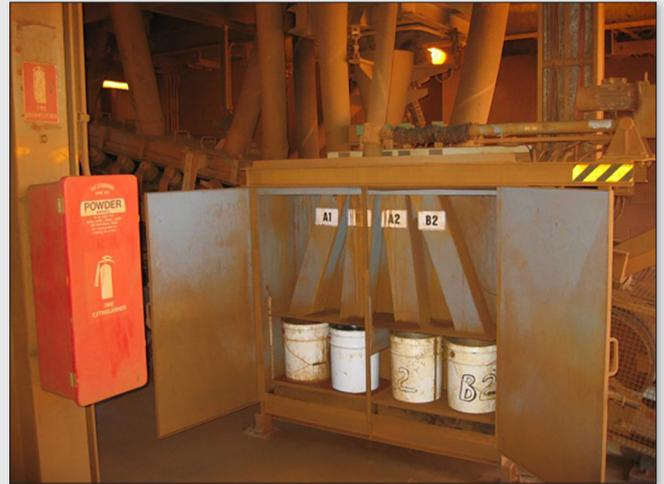
Figure 17. Duplicate sampling system installed in a sample station.
