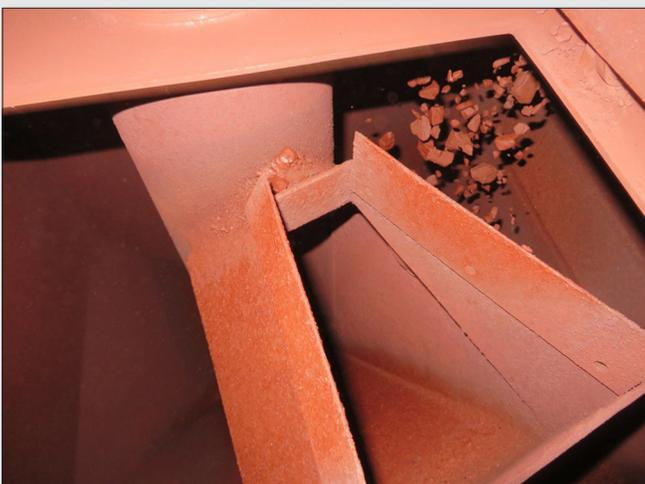
Figure 6. Example of a correctly designed radial Vezin cutter aperture just before interacting with the vertical falling stream of ore.
