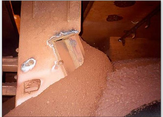
**Figure 10.** Massive reflux from a poorly designed primary cutter aperture at high flow rates.
