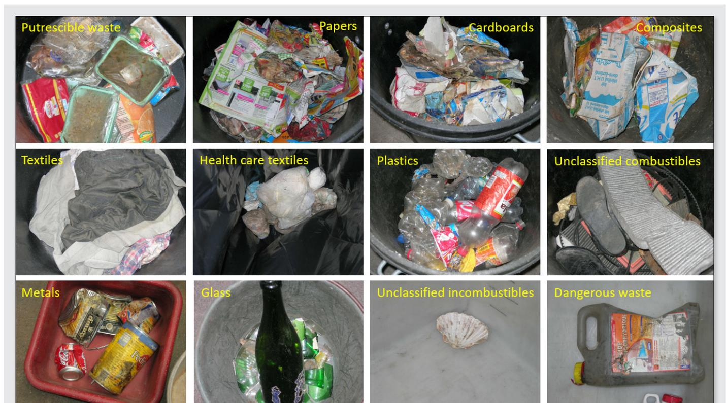
Figure 4. Example of coarse elements (>100mm) after sorting.
