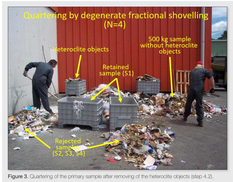
Figure 3. Quartering of the primary sample after removing of the heteroclite objects (step 4.2).
