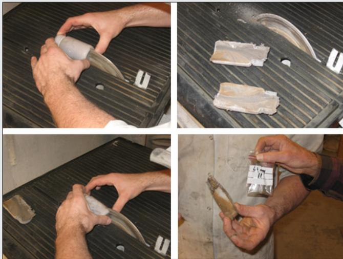
**Figure 7.** Two-stage mass reduction of frozen sample bottles. First cutting is a 50/50 split, followed by a further slice of one of the randomly selected half cores produced, resulting in a 10–15% final sub-sample mass, which is guaranteed to be representative of the original container content in the vertical dimension irrespective of the degree of possible residual segregation present.
