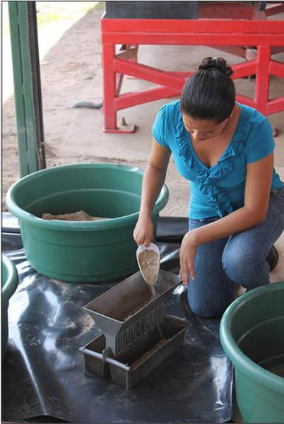
**Figure 5.** Loading the project riffle splitter (kindly provided by GEUS). Sub-sampling is made effective by the fact that the sample to be split does not need to be split all in one, but can be subjected to riffle-splitting in an intermittent loading process.<sup>7</sup>
