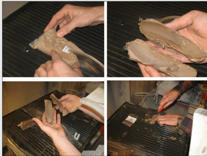
**Figure 8.** Three-stage mass reduction of frozen sample bag content. All cuts are vertical slices again resulting in a 10–15% final sub-sample mass, which is guaranteed to be representative of the original container content in the vertical dimension irrespective of the degree of residual segregation present.
