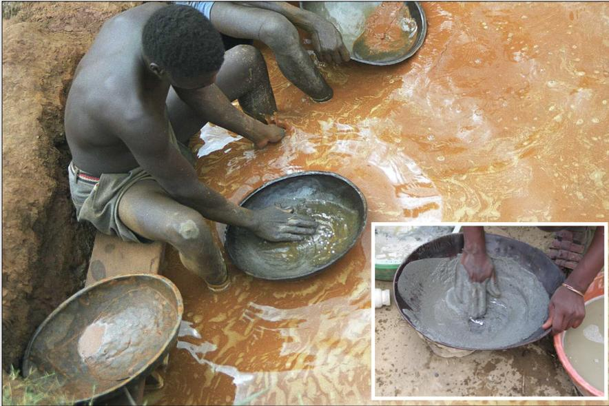
Figure 3. Hand-mixing mercury with milled gold ore (Tanzania).
