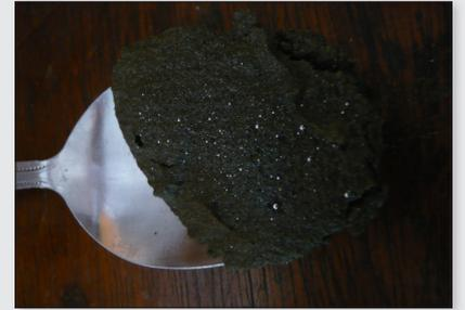
Figure 5. Mercury flour (droplets) in a spoonful of tailings (Philippines).
