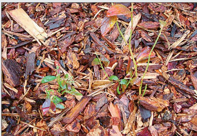
**Figure 2.** Typical fresh wood chips characterised by significant proportion of bark and foliage. Grab-sampling of this type of material will give rise to severe sampling errors (FSE + GSE) if not guided by proper TOS-compliant principles. Add hereto Incorrect Sampling Errors (ISE) if not considered.
